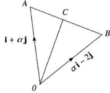
$$\begin{aligned}\vec{OC} &= \vec{OA} + \vec{AC} \\ &= \vec{OA} + \frac{1}{3}\vec{AB} \quad (5) \\ &= (\mathbf{i} + \alpha\mathbf{j}) + \frac{1}{3}[(\alpha - 1)\mathbf{i} - (\alpha + 2)\mathbf{j}] \quad (5) \\ &= \frac{1}{3}[(\alpha + 2)\mathbf{i} + 2(\alpha - 1)\mathbf{j}]\end{aligned}$$
