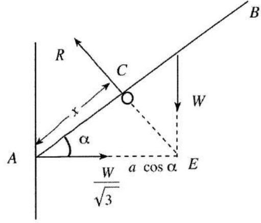
$$\overset{C}{\curvearrowright} \frac{W}{\sqrt{3}} \times x \sin \frac{\pi}{6} = W \times (a - x) \cos \frac{\pi}{6} \quad (5) \quad \text{அல்லது } x = AE \cos \alpha$$
