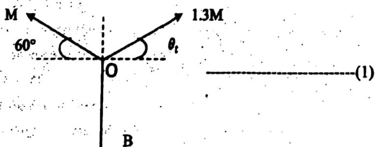
Using Lami's theorem at point O
